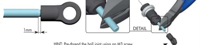
HINT: Pre-thread the ball joint using an M3 screw.
