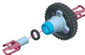
Slide #309319 spacer onto #305131 outdrive shaft.
